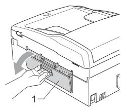
3 Clean the Paper Pick-up Roller (1) with isopropyl alcohol on a cotton swab.
